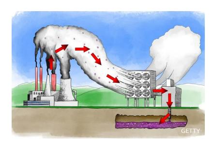
Carbon capture technology filters CO<sub>2</sub> from the air and stores it underground
